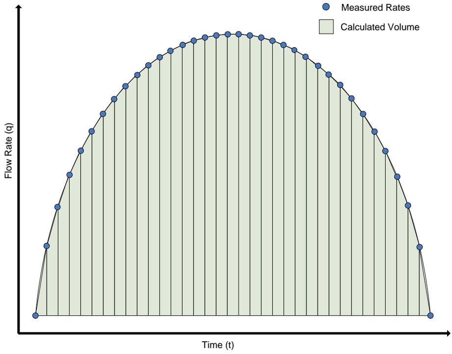
The diagram above illustrates the cumulative volume calculated by using a Trapezoidal volume integration method.
