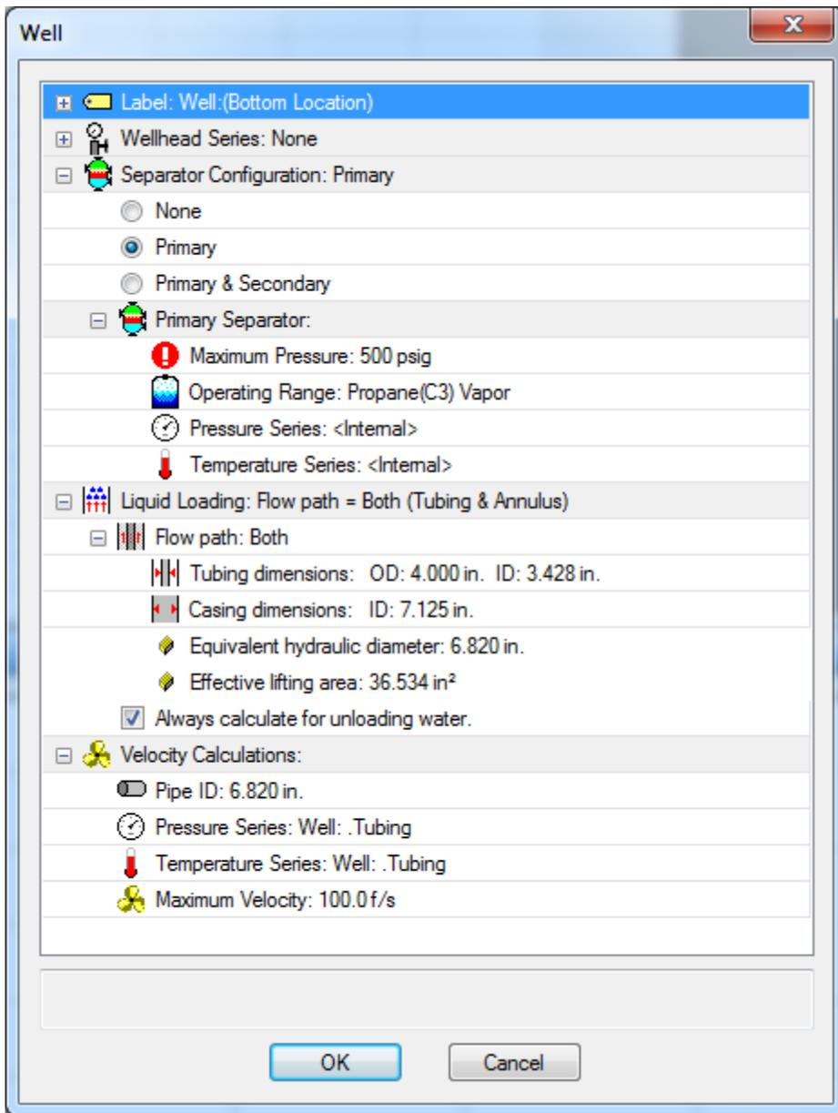
Well configuration dialog contains configuration properties for wellhead series, test separators and monitors for liquid loading and in-situ mixture velocity. The options available are detailed as follows:
