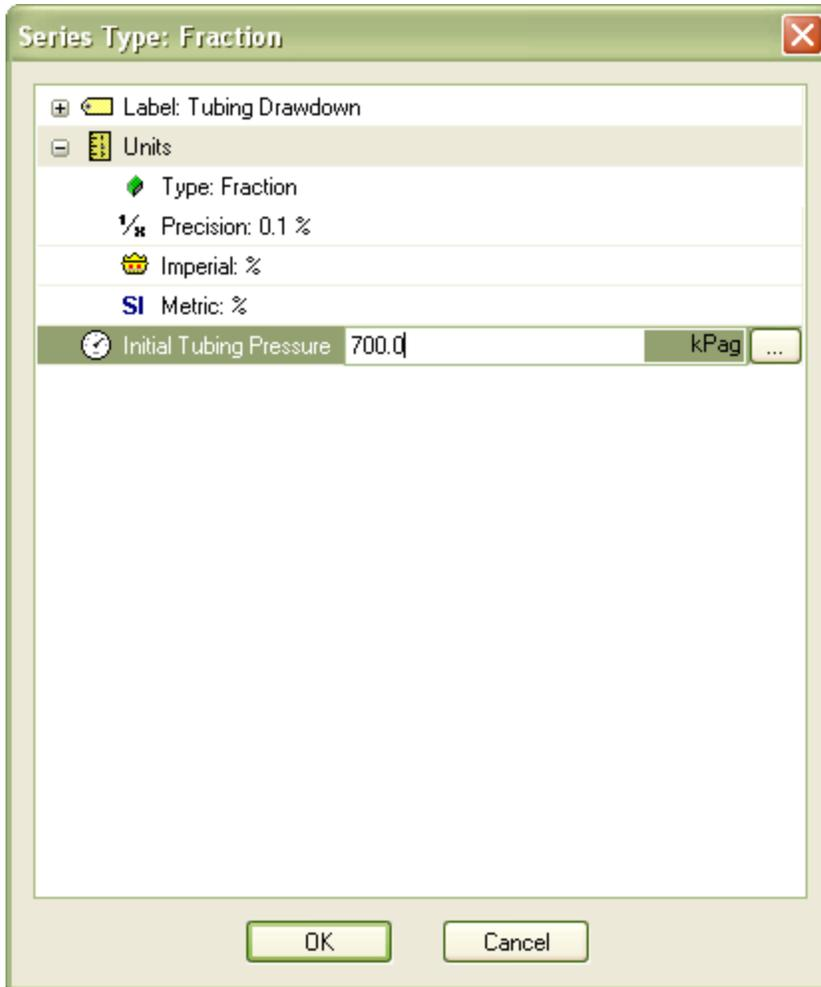
*The tubing and casing drawdown series require an initial pressure. The initial pressure is entered in the series property dialog, for each drawdown series.*
