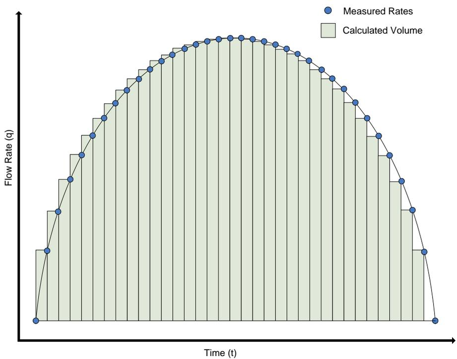
The diagram above illustrates the cumulative volume calculated by using a Rectangular volume integration method.
