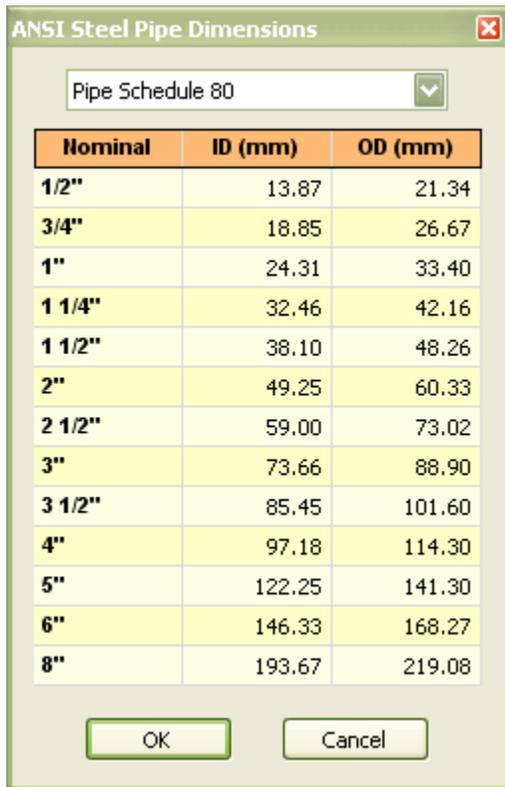
The image shows a dialog box titled "ANSI Steel Pipe Dimensions" with a close button (X) in the top right corner. At the top, there is a dropdown menu currently set to "Pipe Schedule 80". Below this is a table with three columns: "Nominal", "ID (mm)", and "OD (mm)". The table lists nominal pipe sizes from 1/2" to 8" and their corresponding internal and external diameters in millimeters. At the bottom of the dialog, there are two buttons: "OK" and "Cancel".
