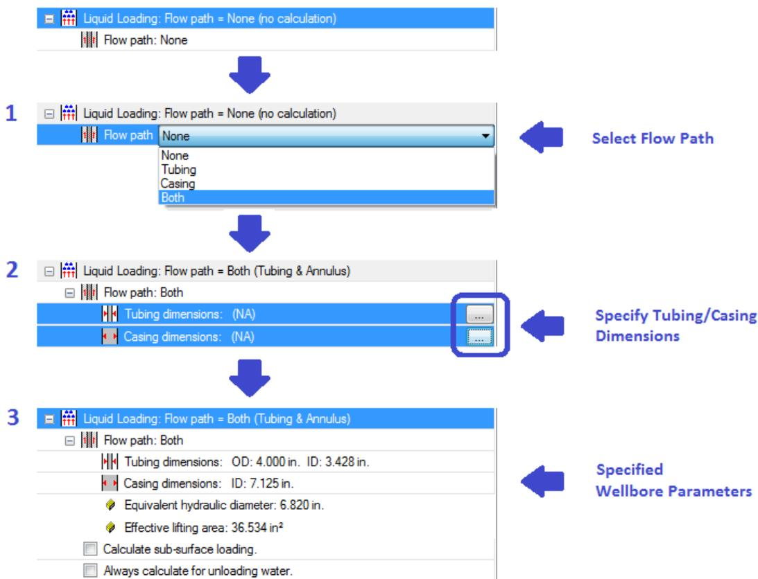
Once the well flow path and pipe dimensions have been entered, two calculated entries (Equivalent hydraulic diameter and Effective lifting area) will be displayed along with the following options:
