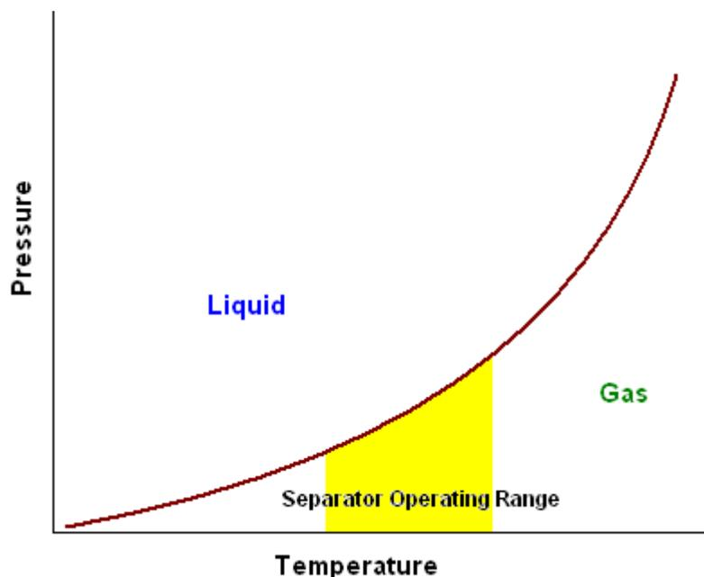
Pressure temperature diagram illustrating the separator operating range.
