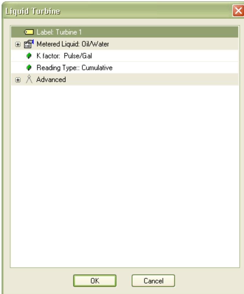
The Liquid Turbine meter contains the following configuration variables:
