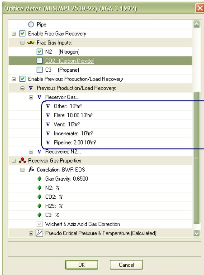
Previous production breakdown for a gas meter
